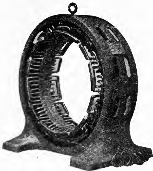
FIG. 14—DETAIL VIEW OF THREE-PHASE CONCENTRIC WINDING
